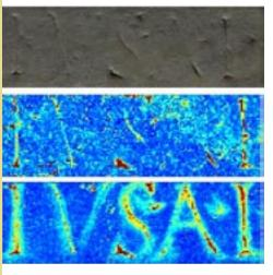
In this group of scanned letters, the top panel is a photographic image. The middle panel is iron fluorescence, which becomes very weak in areas that have been significantly worn away. The bottom panel is lead fluorescence. Even in areas that have been significantly weathered, the fluorescence is strong enough to clearly read the text.
