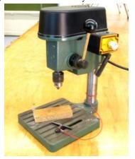
Because these machines are only a foot high, they're limited as to the size of workpieces that can fit into the machine and the size of the drill bits you can use. But I've had no problems with drill bits up to about 3/16" (4.5mm), even drilling steel.
